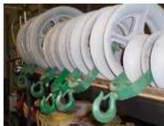
E Greenlee pulleys hook sheaves
